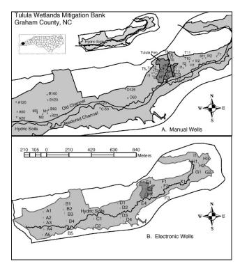
Figure 1. Maps showing location of manual wells (A) and electronic wells (B) used to assess site hydrology of the restored Tulula stream channel in Graham County, North Carolina. Manual wells A120, B160, and B120 were destroyed during site restoration and not replaced. Stream flow is from east to west. The light gray areas of the maps represent the extent of hydric soils on site. The solid black line in Map A near Tulula Fen represents a cross-section of wells illustrated in Figure 5.
